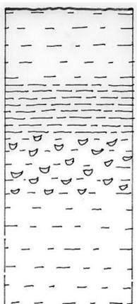
**Underlayers:** Alternating silt & clay with shells. No greywacke stones but some small pieces of wood.
