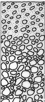
**Underlayers:** Sand & rounded greywacke river stones on larger greywacke river stones (2-100mm rounded)
