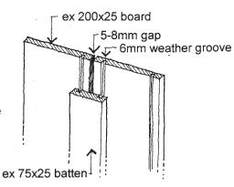
The same effect can be achieved quite economically using sheet materials, like plywood or fibreboard, which looks appropriate with closely spaced battens fixed over and generous thickness architraves around windows and doors. Dark, corrugated *Onduline* can also look most appropriate with weathered timber facings. A weatherboard texture can also be achieved with *Hardies Weatherboards*.
