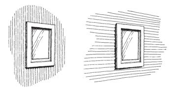
Coloured corrugated steel fits in well on roofs and walls, with vertical or horizontal profile
